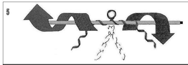
Continue wrapping the legs of the Tangent Support around the SRR making sure that the gaps between the legs are evenly spaced. Do not apply the last two pitches.
