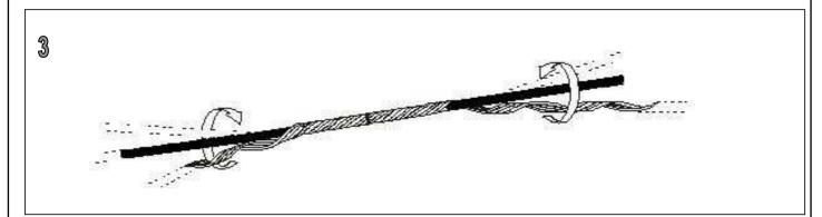
To complete application of the SRR, use both hands to wrap subsets simultaneously into position. First wrap one end, then wrap the other end. To assure a strong reinforcement, MAKE SURE THAT RODS ARE NOT CROSSED, AND THAT ALL RODS ARE EVENLY SPACED.
