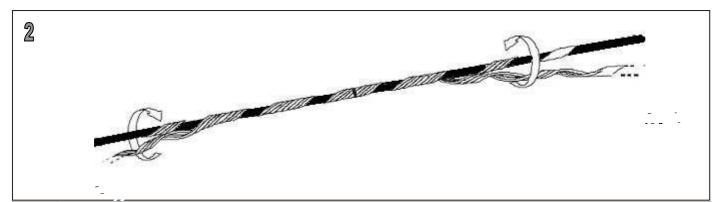
Align the center mark of a second subset with the first subset. Wrap the second subset on the cable two or three times leaving the ends loose. Apply remaining subset as outlined above.
