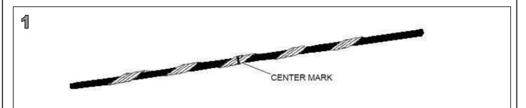
Begin at the center mark of the subset and wrap the subset by pulling the rod legs up and away from the cable. Wrap the rods of the first subset completely around the cable.
