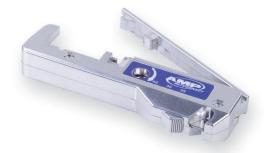
AMP-TWIST SL TOOL is a high performance shielded (STP) termination tool, capable of terminating cable in less than 60 seconds. SL TOOL terminates all types of SL Jacks (110C, AMP-TWIST 6S, AMP-TWIST  $6_AS$ ). It strips cable, marks foil, terminates and cuts eight conductors at once. SL TOOL maintains twisted pair integrity while producing reliable connections every time.
