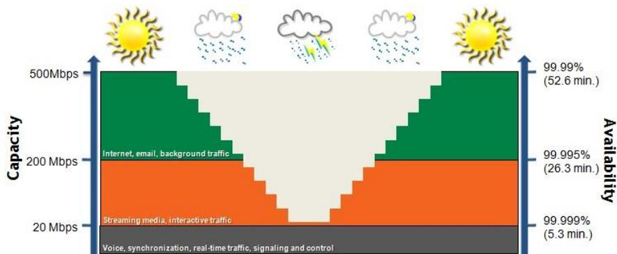
Figure 1-1 Hitless Adaptive Bandwidth, Coding and Modulation
