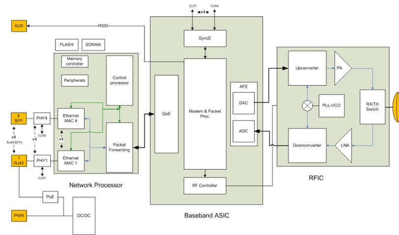
Figure 1-2 EH-1200TX (TDD) Functional Block Diagram
