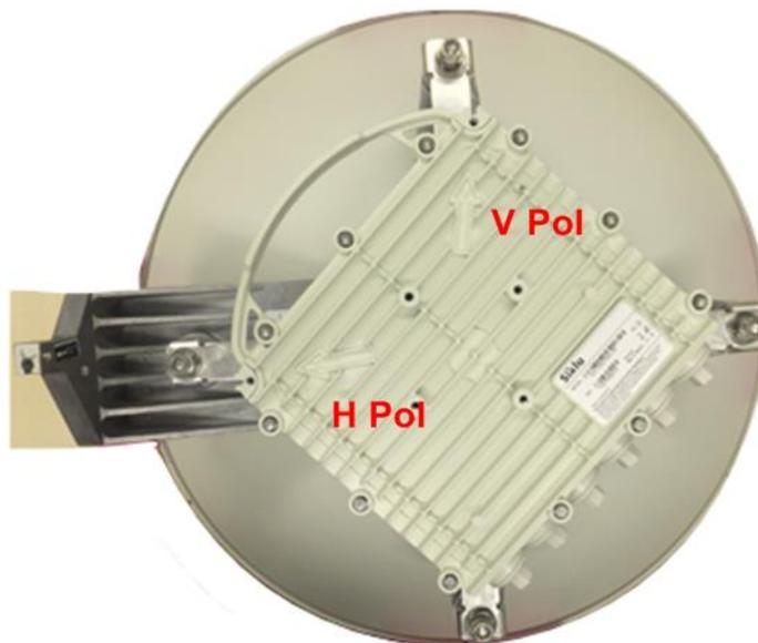
Figure 2-4 EtherHaul ODU installed on 2ft Antenna
