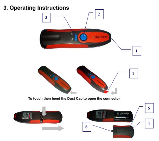
To press to release Linchpin then to push To open Battery Lid to change batteries. Battery Lid backward.
