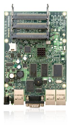
The RB433AH is a more powerful version of the standard RB433. The 128MB DDR will be capable of supporting new RouterOS features coming. The microSD slot supports an additional memory card that can be used for a Dude database and other features to be announced in during Spring '08.
