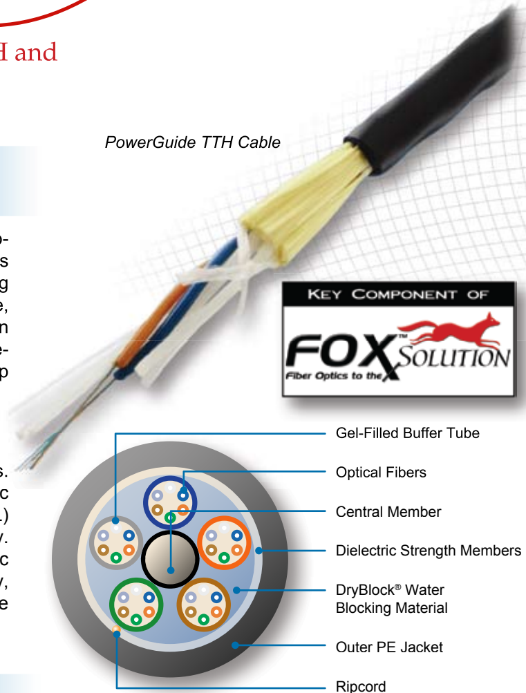
PowerGuide TTH Cable Cross-Section
