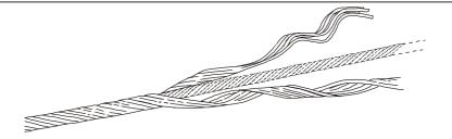
To ease application split the legs on the last two pitches. Make sure all rod ends are snapped into place. Do not use a tool to snap in rod ends.
