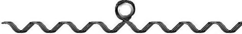
4 The Tangent Support is supplied with the thimble inserted in its loop. Begin application by wrapping one leg over the SRR starting at the center mark.
