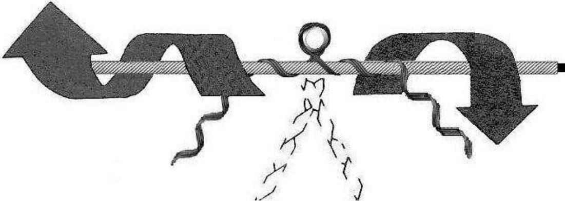
5 Continue wrapping the legs of the Tangent Support around the SRR making sure that the gaps between the legs are evenly spaced. Do not apply the last two pitches.
