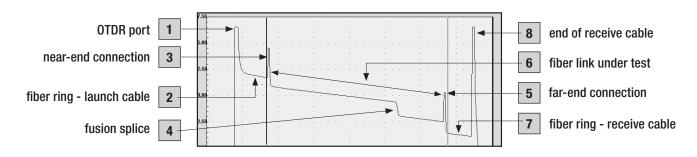
OTDR Trace Made Using Launch And Receive Cables.
