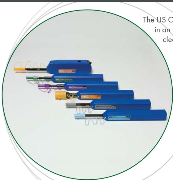
The US Conec IBC™ Brand Cleaners are mechanical cleaning tools designed to clean connectors residing in an adapter or faceplate and unmated connectors. The IBC™ Brand Cleaning tools use a novel dry cleaning strand to gently sweep and lift away dust and residues from the connector end face.
