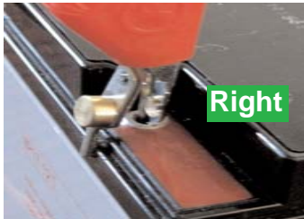
Insert clips fully inside battery terminals
