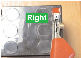
Grip clips tightly around tab terminals
