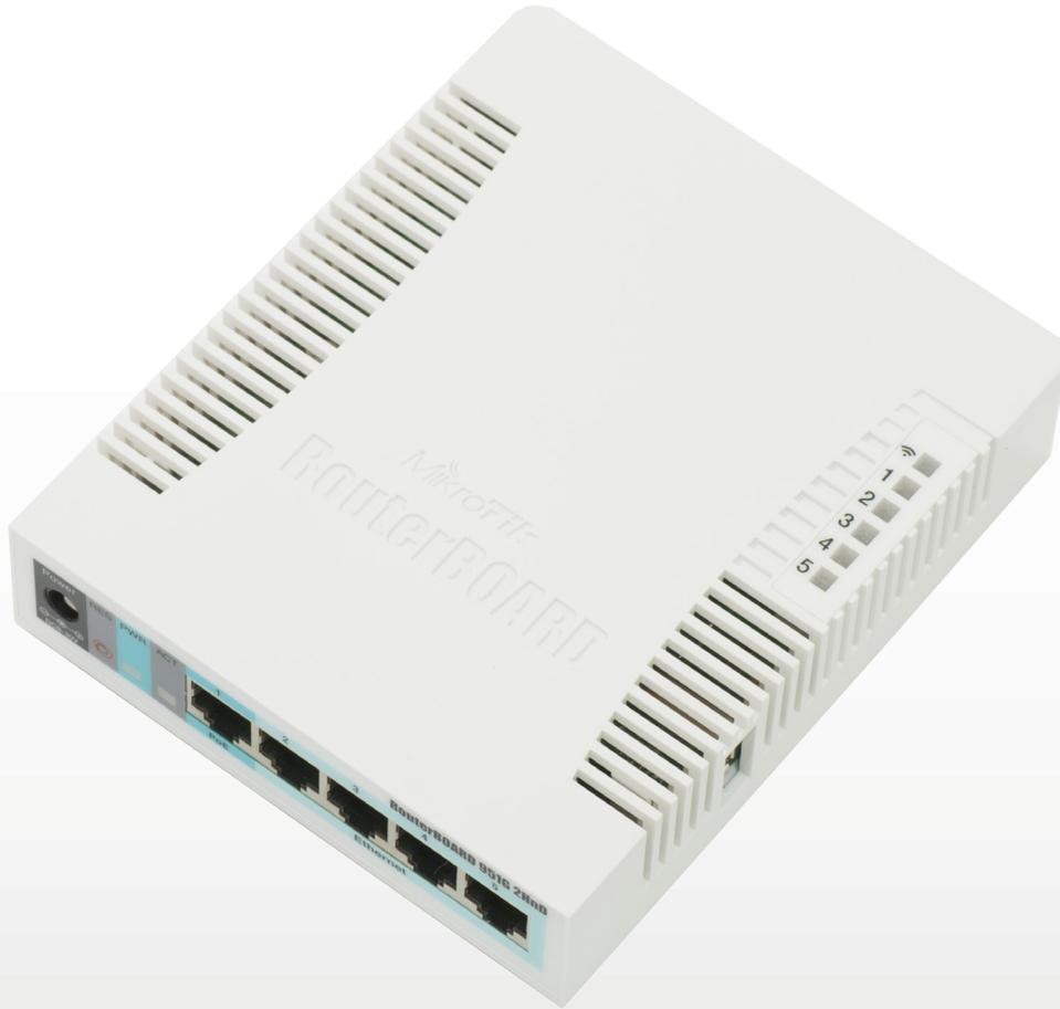
The RB951G-2HnD is a wireless SOHO Gigabit AP with a new generation Atheros CPU and more processing power. It has five Gigabit Ethernet ports, one USB 2.0 port and a high power 2.4GHz 1000mW 802.11b/g/n wireless AP with antennas built in.
