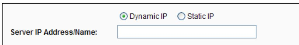
Select **Static IP** if IP Address/ Subnet Mask/ Gateway and DNS server address have been provided by your ISP. Then please enter server IP address or domain name provided by your ISP, and also enter the corresponding parameters.
