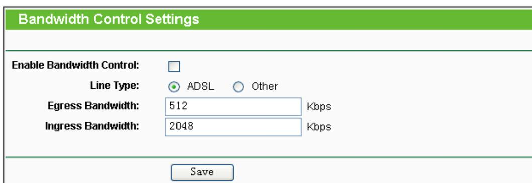
A screenshot of the 'Bandwidth Control Settings' web page. The title bar is green with white text. Below the title bar, there is a section for 'Enable Bandwidth Control' with an unchecked checkbox. Underneath, there is a 'Line Type' section with two radio buttons: 'ADSL' (checked) and 'Other'. Below that, there are two input fields: 'Egress Bandwidth' with the value '512' and 'Kbps', and 'Ingress Bandwidth' with the value '2048' and 'Kbps'. At the bottom of the form is a 'Save' button.
