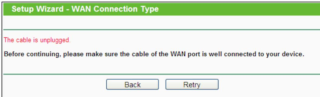
4. If you select **Auto-Detect**, the router will automatically detect the connection type your ISP provides. Make sure the cable is securely plugged into the Internet port before detection. The appropriate configuration page will be displayed when an active Internet service is successfully detected by the router.
