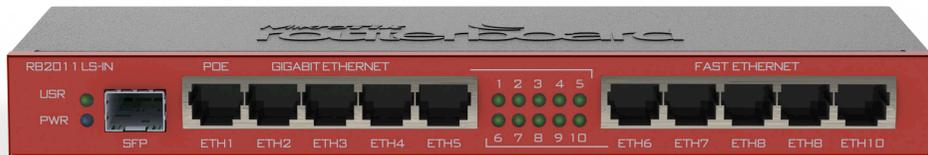
The RB2011LS has 11 ports: Gigabit SFP cage and five Gigabit Ethernet ports that can be switched together providing affordable wire-speed Fiber-to-Copper converter, and additional five Fast Ethernet ports. Board can be powered by power jack or PoE.
