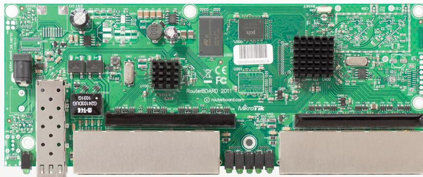
It's powered by the new Atheros next generation 600MHz 74K MIPS network processor and has 64MB of RAM and a Level4 RouterOS license. RB2011LS-IN comes with an indoor case, optional wall mount kit is available separately.
