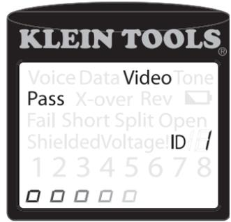
**Coax Cable Properly Wired with ID Remote #1:** The #1 ID remote is used to terminate a properly wired coax cable. The video test passes, ID #1 is detected, and the "o"s across the bottom of the screen show that the tester is running tests continuously.
