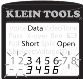
**T568A Cable with a Short and an Open:** The 1-2 pair pins are shorted together and the 7-8 pair is open. The pins with the errors are flashing. Dash lines (-) on the bottom (remote) display line indicate the short, while no numbers on the bottom line indicate the open pair.
