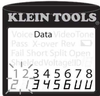
**T568A Cable with a miswire and unrecognized continuity:** 1 and 2 pins on the VDV Scout® Pro 2 are connected to pins 2 and 1 at the remote-end. The pins with this error are flashing. The "U" for the remote pin numbers indicates an unrecognized continuity was detected that is neither a short or open. An ID remote connected to the VDV Scout® Pro 2 when in cable test mode would also show this error.
